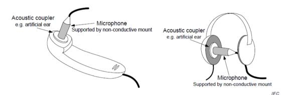
NOTE 1 The microphone is connected via the cable to a suitable amplifier.
