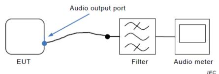
The filter is the audio filter specified in G.6.1 and is typically incorporated into the audio meter. Additional filtering might be necessary to ensure that the RF disturbance signal does not interfere with the measurement.
