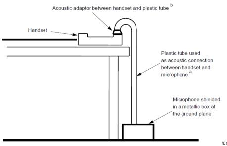
NOTE This set up is suitable for radiated immunity testing. See G.6.3.
