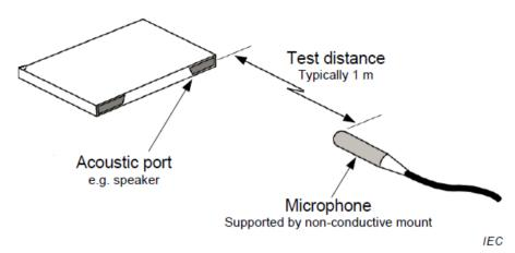
The microphone is connected via the cable to a suitable amplifier. Ensure that there is minimal acoustic loss between EUT and microphone.
