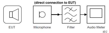
The filter is the audio filter specified in G.6.1 and is typically incorporated into the audio meter. Additional filtering might be necessary to ensure that the RF disturbance signal does not interfere with the measurement.
