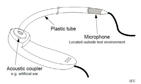
NOTE 1 The microphone is connected via the cable to a suitable amplifier. NOTE 2 This setup is suitable for radiated immunity testing. See G.6.3
